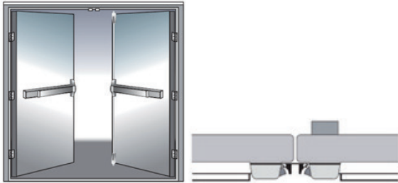
Mortise Lock Device & SVR Device Combination – same direction. Overlapping astragal is not required, but coordinator required with a standard ANSI strike.
