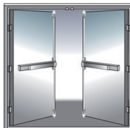
SVR and Three-Latching Device combination – same direction. Overlapping astragal is not required, but coordinator required with a double door strike.
