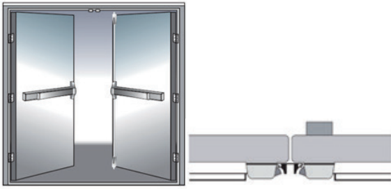
Rim Device and SVR or CV Device combination-same direction. Overlapping astragal is not required, but coordinator required with a double door strike.
