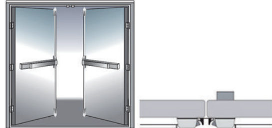
Two Surface Vertical Rod (SVR) or Concealed Vertical Rod (CVR) – same direction. Overlapping astragal is not required.
